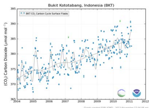
Figure 2. Trend of CO 2 concentration at Bukit Kototabang in 2004-2011.
