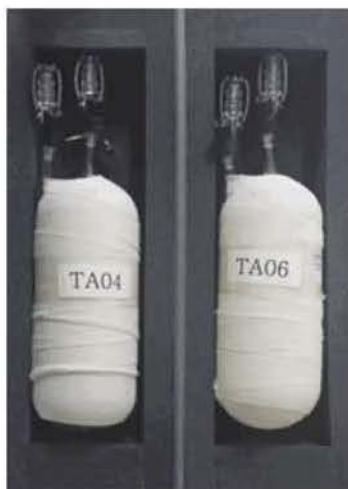
Figure A5. Glass flasks. In order to block stray light, a scrap is wrapped.
