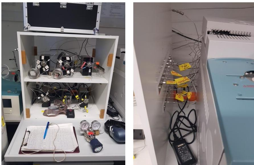
Figure 5. The valve system (left) and the connections to GC (right)
