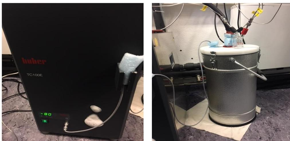
Figure 4. The thermoregulator TC100 E (left) and the cooling trap (right)
