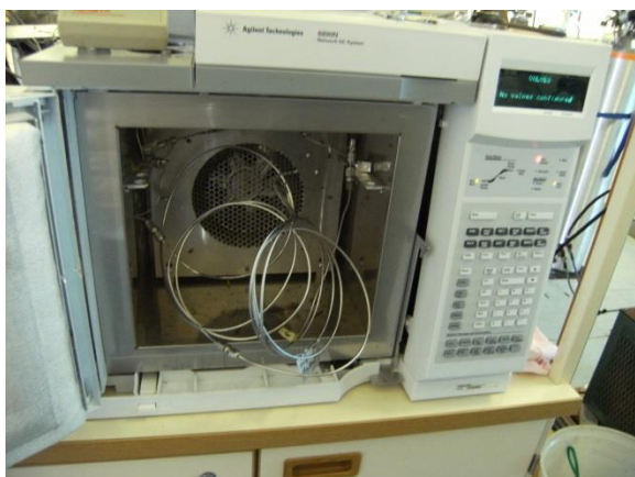
(a) Previous column setting condition (Heysep-Q 8+6 ft, 1/8")
