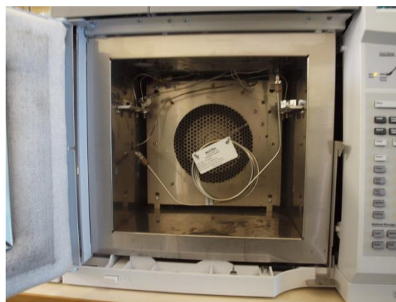
(b) Current column setting condition (Porapa-Q 12 ft, 1/8")
