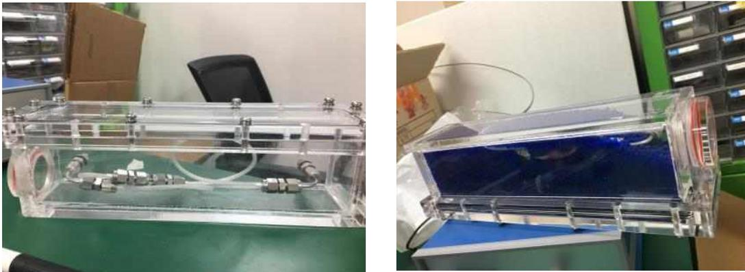
Fig. 2.4.3. The picture of Nafion membrane tube(24" length) installed in acrylic box (left), and it filled with chemical dryer of silica gel (right).
