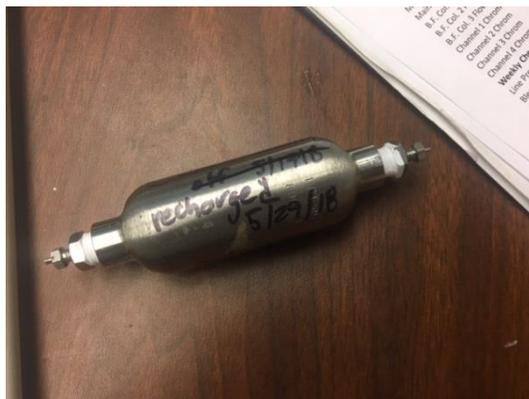
Figure 4. The chemical trap filled with  $\text{Mg}(\text{ClO}_4)_2$  for drying air.
